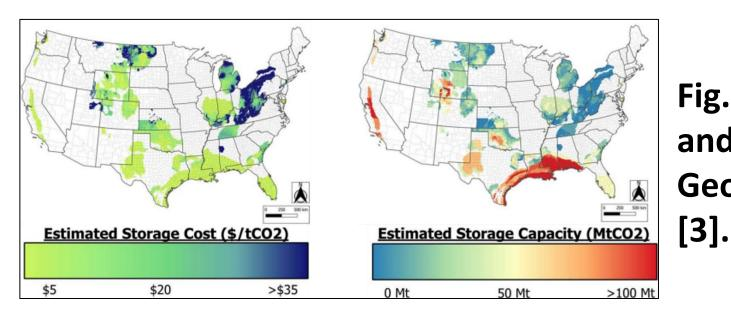
Fig. 1: Geospatial Cost Capacity of Geologic CO<sub>2</sub> Storage
