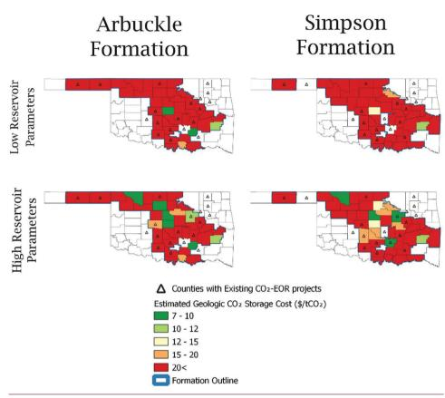
Figure 3. Estimated geologic CO<sub>2</sub> storage costs for the Arbuckle and Simpson saline formations in Oklahoma.
