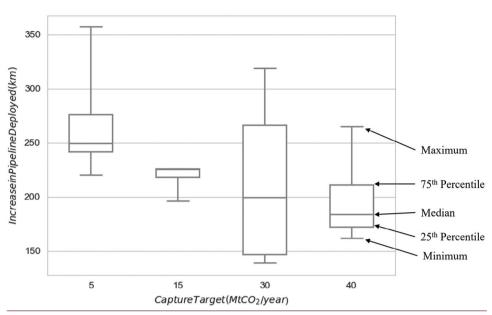
Figure 6. Distribution of the increase in pipeline deployed for between scenarios in which  $CO_2$  can be injected in any county with geologic  $CO_2$  storage and only counties with geologic  $CO_2$  storage resources with  $CO_2$ -EOR operations. Distributions are across all scenarios of geologic parameters and  $CO_2$  capture costs.
