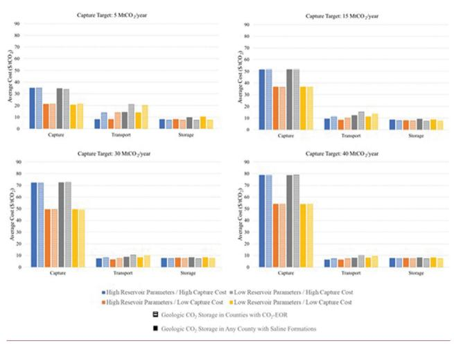
Figure 5. Breakdown of average cost for each capture target and combination of scenarios.
