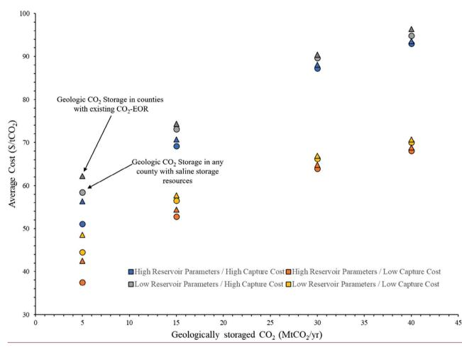
Figure 4. Average cost of the CCS network when geologic  $CO_2$  storage can occur in (circles) any county with saline storage resources and (triangles) only in counties with existing  $CO_2$ -EOR projects.
